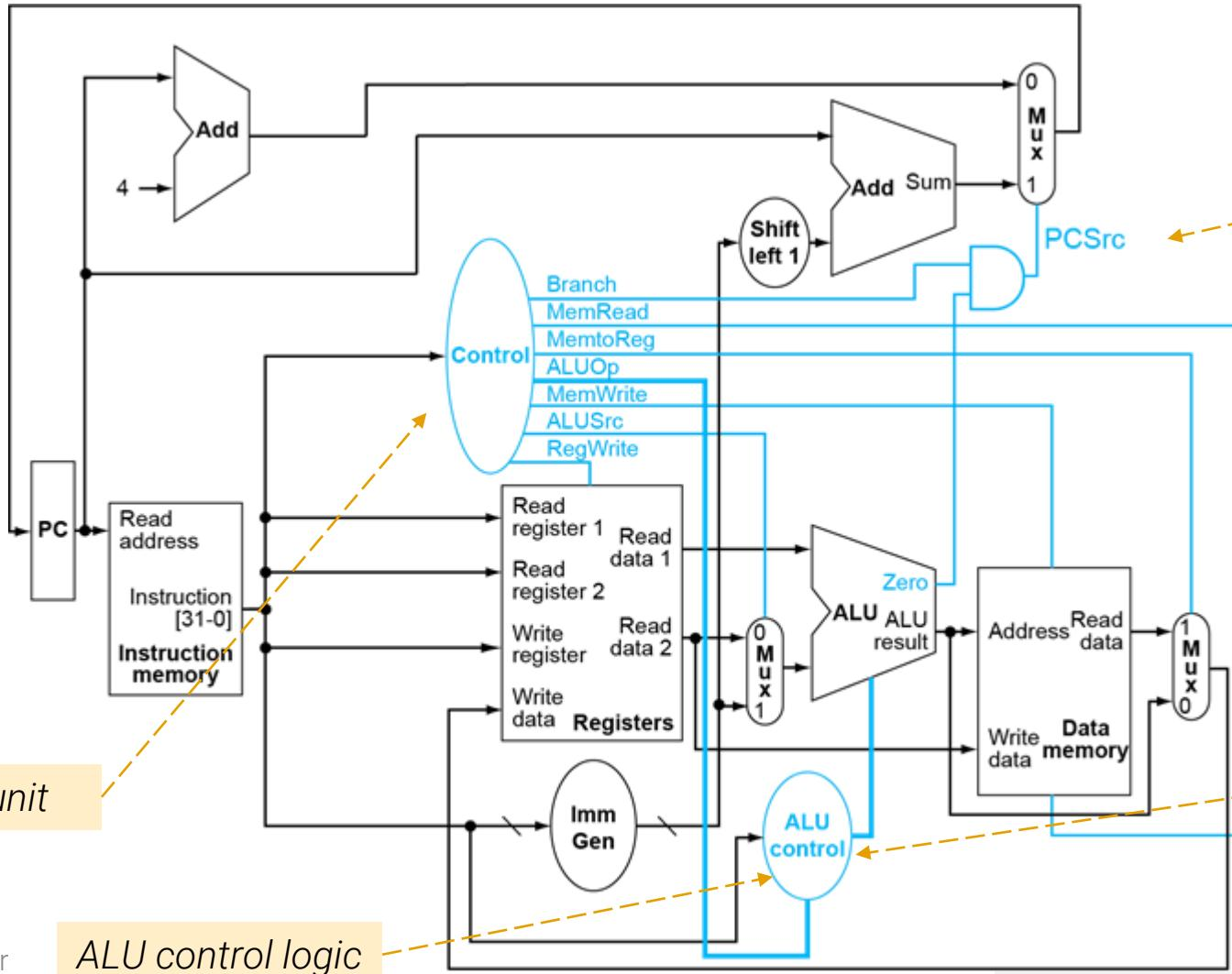
Note: The control unit can set all but the **PCSrc** control signal based solely on the **opcode** and **funct** fields of the instruction.
